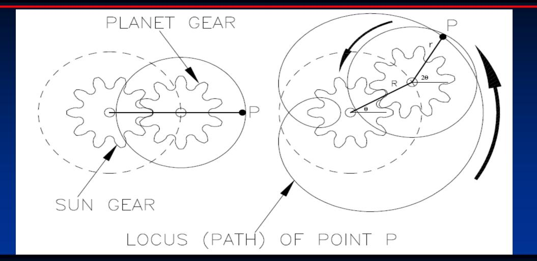
The coils are subject to double rotation in what is known as planetary motion (like Earth rotation, it rotates own axis as rotates around the sun, this is defined as "J" type.
