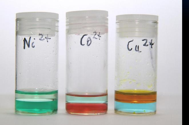
Ni<sup>2+</sup> strongly prefers the water phase Co<sup>2+</sup> is more soluble in the water phase than ionic phase Cu<sup>2+</sup> prefers the ionic phase
