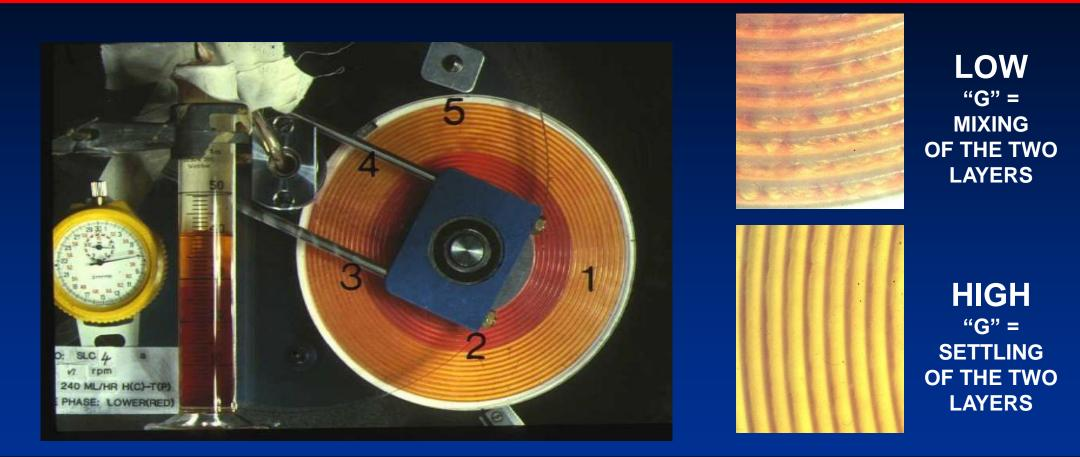
Imagine on Earth, at 1 "G" fixed wind causes 10 foot wave in ocean / water interface. Imagine same wind, same ocean, **<u>BUT</u>** 200 "G"? NO WAVE / NO MIXING. At 0.1 "G" FORCE OCEAN & AIR RAPIDLY MIXED.
