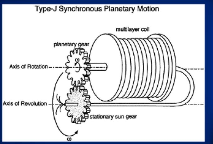
The flying leads go through both the axis of rotation and the axis of revolution
